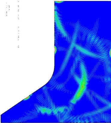
*Sound reflections in the wing to fuselage fitting*
